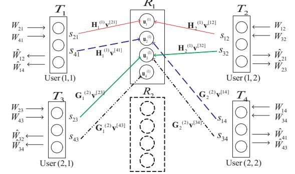
Fig. 3. Two-way relay X channels with signal space alignment during the MAC phase
