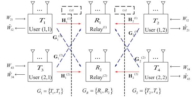
Fig. 2. MAC phase of two-link two-way relay channels and its cut-set region
