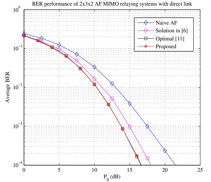
Fig. 4. BER performance comparison for various relay transceiver designs with QPSK constellation as a function of  $P_0$
