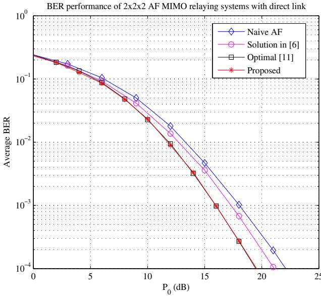
Fig. 3. BER performance comparison for various relay transceiver designs with QPSK constellation as a function of  $P_0$
