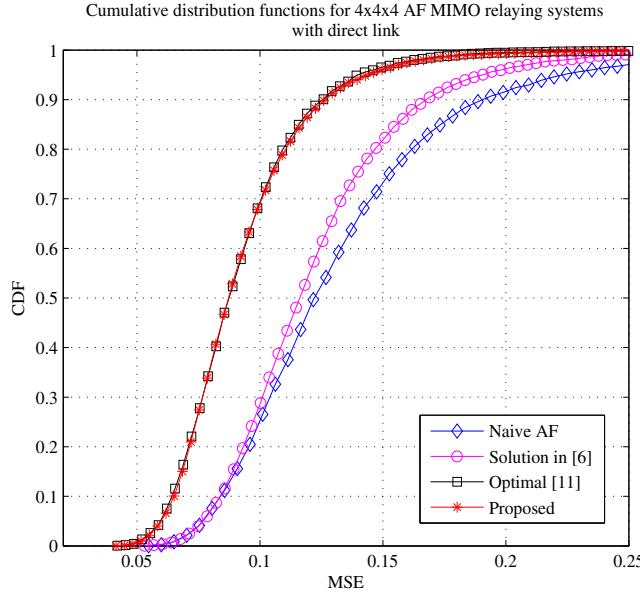
Fig. 2. CDFs of the instantaneous MSE for various relay transceiver designs at  $P_0 = 20$  dB
