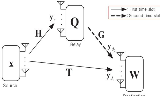
Fig. 1. System description for an AF MIMO relay network with direct link
