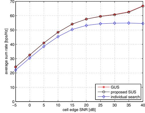
Fig. 4. Average sum rate performance of a seven cell network with asymmetric system configurations
