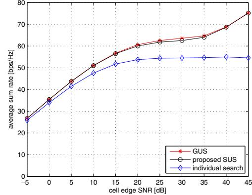
Fig. 2. Average sum rate performance of a seven cell network with  $N_t = 4$  and  $K = 10$
