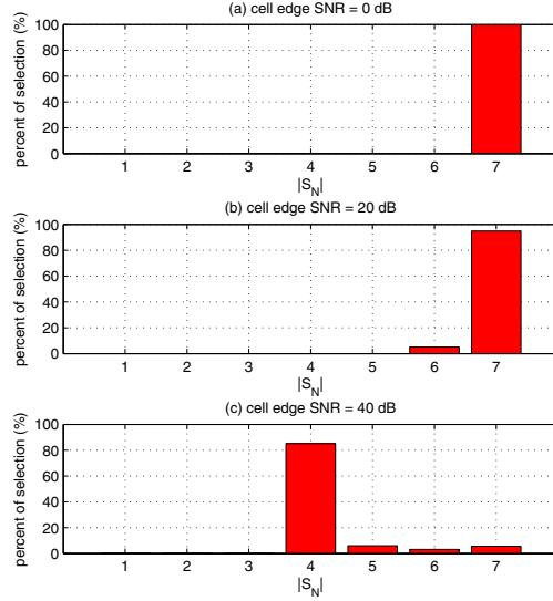
Fig. 3. Histogram of the size of active users  $|S_N|$  for SUS.
