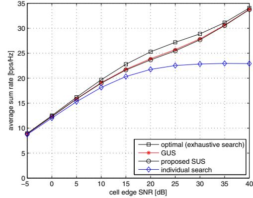
Fig. 1. Average sum rate performance of a three cell network with  $N_t = 2$  and  $K = 3$
